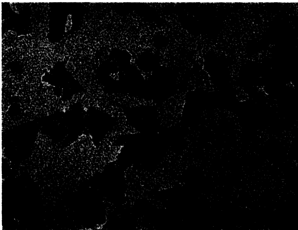
FIG. 8. Electron micrograph of a 50 Å thick film after calcination in air at 250°C for 45 hr. The particles are distributed.
